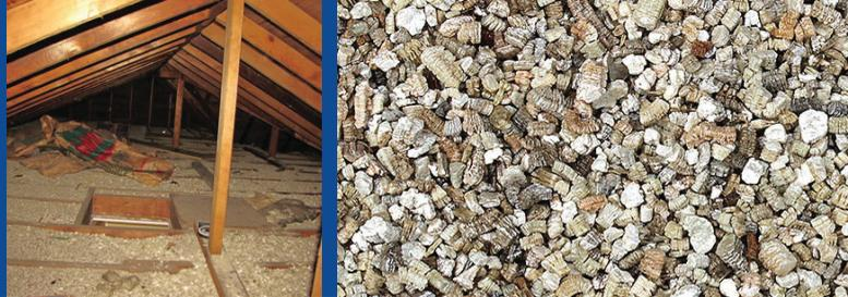
**Vermiculite is a naturally-occurring mineral composed of shiny flakes which resemble mica.** When heated to high temperature, the flakes expand into a light-weight, fire-resistant, and odorless material used in numerous products, including insulation for attics and walls.
